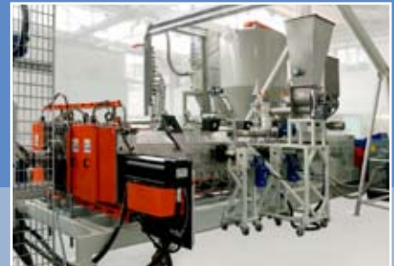
Micro-batch feeders on top of extruder
