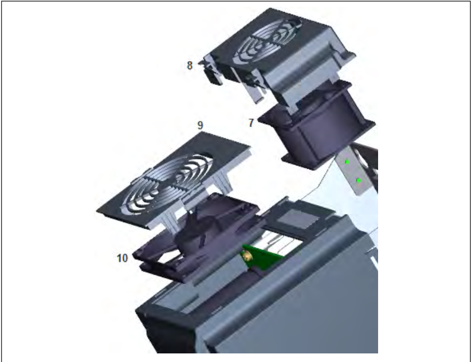
Fig. 16-3: Disassembly of fan
