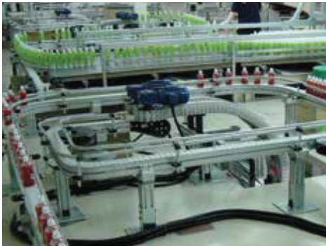
Bottle Production Line Intergrated with Gripper Conveyor
