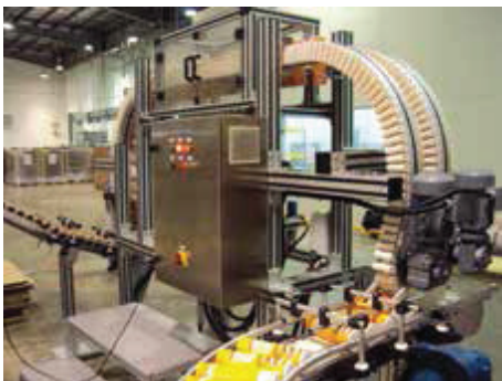
Gripper Conveyor System Integrated with Can Cleaner to Remove Dust and Particles from Can.
