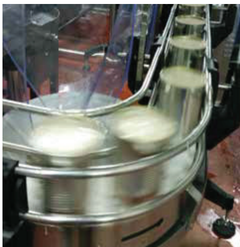
Stainless Steel Conveyor for Wet Environment
