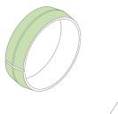
Lubricant with a high MoS<sub>2</sub> content must be applied again to the taper surfaces of the thrust rings and the inner ring.
