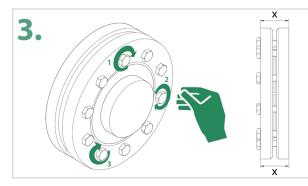
Hand-tighten 3-4 screws. Make sure that the discs are aligned parallel to each other. (x)
