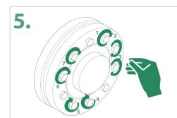
Subsequently apply all other screws to the discs by hand.
