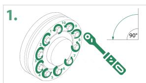
Loosen the screws of the shrink disc one after the other in several turns. Use a maximum of a quarter turn.
