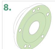
The contact surfaces of the flanges must be cleaned, grease-free and dry.
