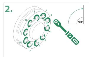
Loosen the screws of the shrink disc one after the other in several turns. Use a maximum of a quarter turn.
