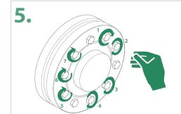
Subsequently apply all other screws to the discs by hand.
