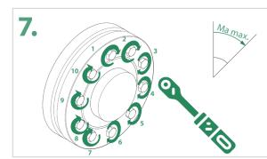
Then tighten the screws to the specified tightening torque in a further 2-3 cycles.
