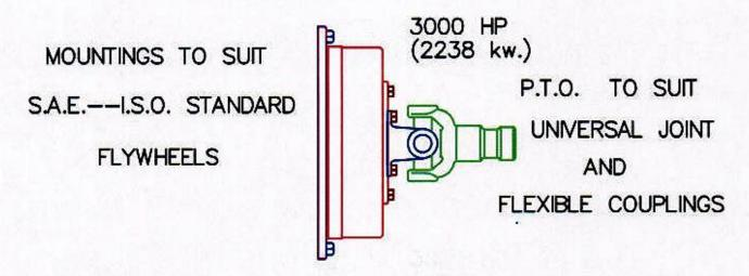
THE "FM" RANGE OF CENTRIFUGAL CLUTCH IS DESIGNED SO THAT THE DRIVING ELEMENTS CAN BE INSPECTED OR REPLACED BY SIMPLY REMOVING DRUM AND RESTING ON DRIVE SHAFT, WITHOUT MAJOR DISASSEMBLY, THE ENGINE AND CLUTCH CAN THEN BE RUN WITHOUT CLUTCH DRUM FOR TESTING PURPOSES.
