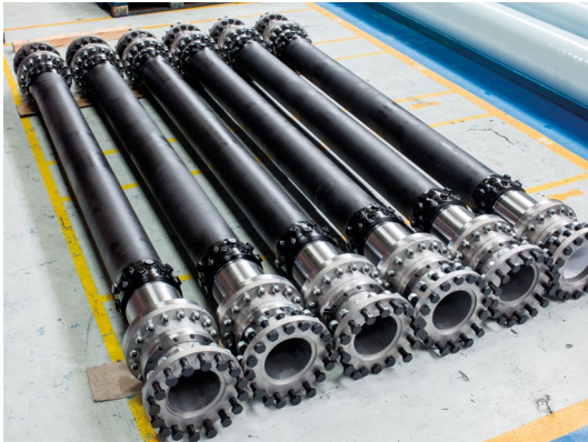
Gear coupling with JCFS carbon fiber shaft
