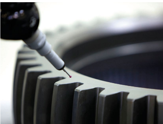
Gear inspection in CMM
