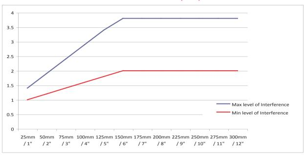
Eg - The spring lip measures 48.5mm and does not appear to be heavily worn, the shaft diameter would be between 49.6mm and 50.3mm (48.5 + 1.1 = 49.6, 48.5 + 1.8 = 50.3). Shaft size is most likely 50mm.
