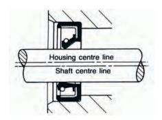
Due to errors machining or excessive build-up of adverse tolerances can cause excessive wear on one side of sealing lip becasue of unilateral loading of lip.
