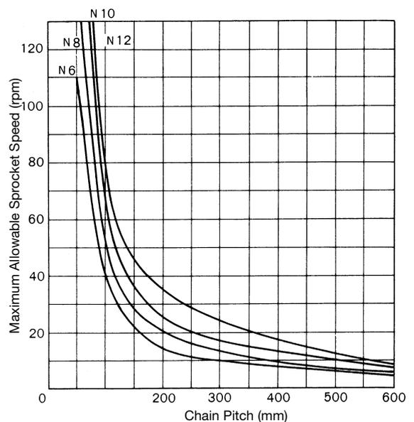
Chain Pitch and Maximum Allowable Sprocket Speed Related
