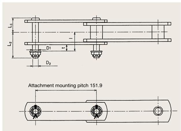
Note: The attachment mounting pitch for the HSS15235 is 151.8mm.
