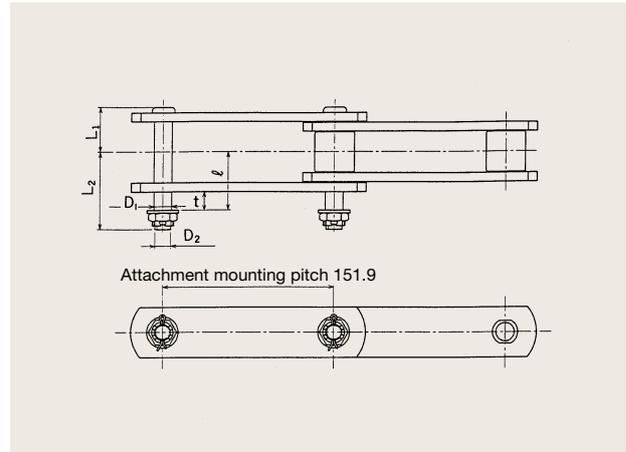
Note: The attachment mounting pitch for the HSC15235 is 151.8mm.
