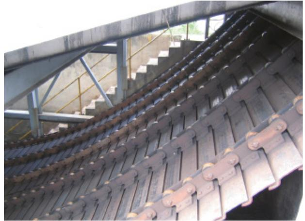
**Cane Feeder and Cane Carrier**
