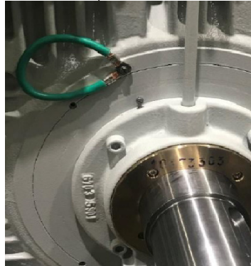
Figure 49 - Metal flexible braid
