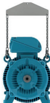
Figure 10 - Use of a spreader beam for lifting
