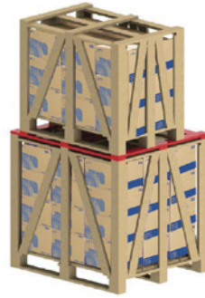
Figure 28 - Use of additional battens for stacking
