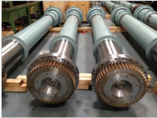
Case carburized gear spindles
