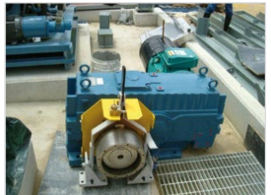
Disengaging gear with lever
