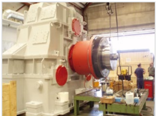
Jaure MTGX-HD-TI-1000 on wind test bench
