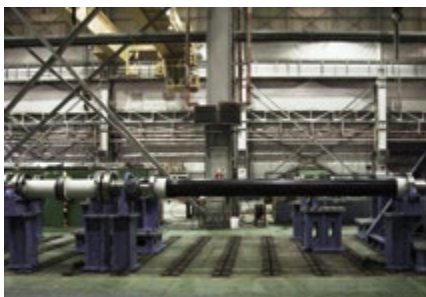
Carbon Fibre Shaft combined with LAMIDISC® coupling.
