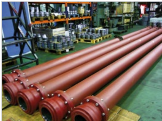
Jaure gear coupling for underwater operation
