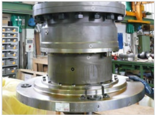
Shear pin type gear coupling
