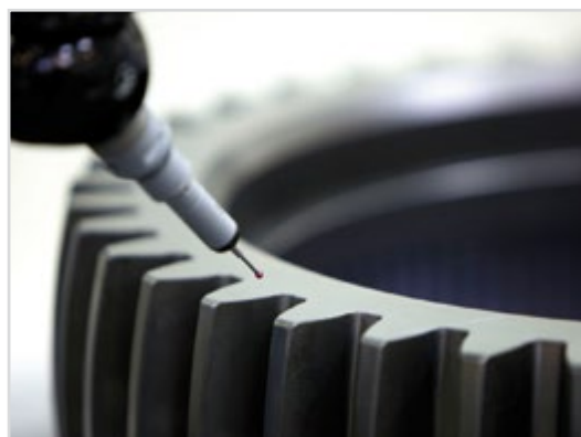
Gear inspection in CMM
