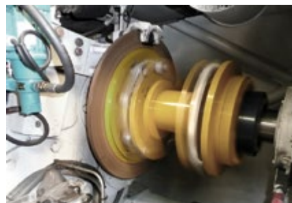
Torque monitoring on wind turbines.
