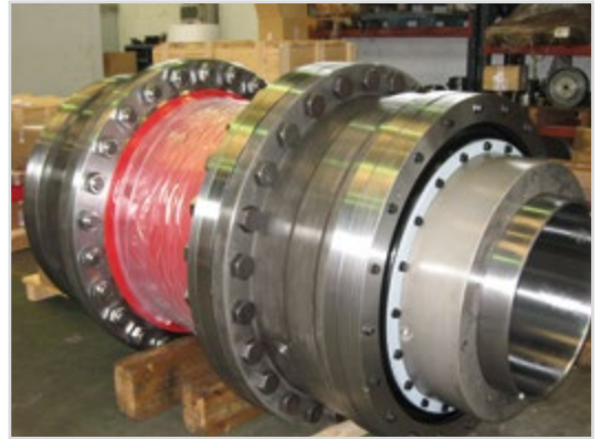
Dredger gear coupling
