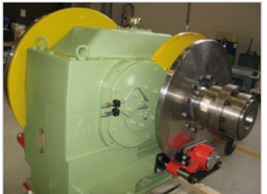
Jaure gear coupling with brake for hoisting
