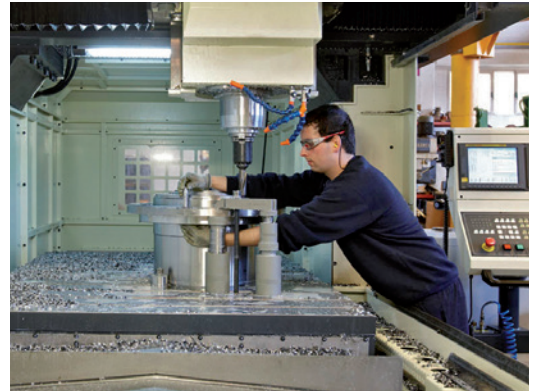
Machining of barrel coupling's hub.
