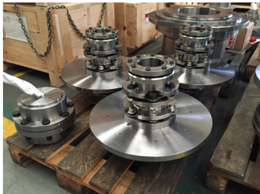
Disc pack configuration with brake disc.
