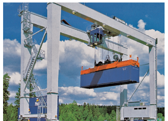
Rubber tyred gantry crane.
