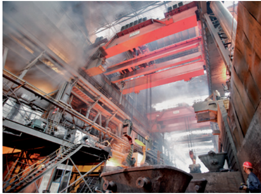
Travelling crane in steel plant.
