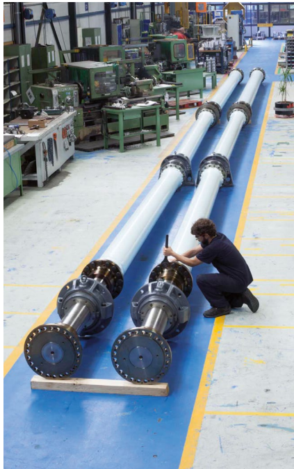
Lamidisc® coupling 505-8 with JCFS-FP Composite Shafts
