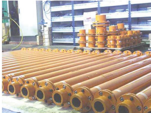
SX type Lamidisc® coupling with long spacers for paper industry
