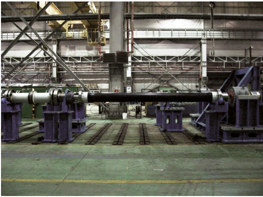
Lamidisc® coupling 605-8 with JCFS composite shafts
