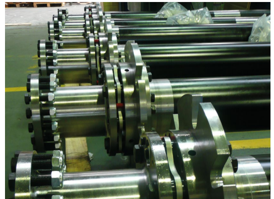
Lamidisc® coupling 410-8 with locking device
