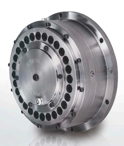
The type RDBK is a centrifugally lift-off sprag RSCI high speed backstop (Please refer to pages 72 to 75) equipped with integral torque limiter. The latter limits the backstop transmissible torque to a value that is factory set-up according to customer request.
