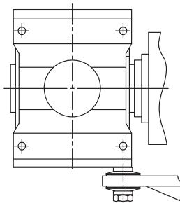
All units can be supplied with elastic constraint, semi-flexible and rigid reaction arrangement.
