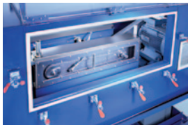
Testing of chain wear elongation behavior on more than 20 testing rigs
