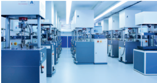
More than 15 pulsers are available for testing dynamic fatigue strength according to different testing methods
