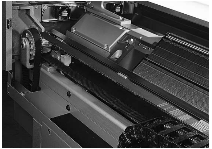
Large Knitting Machine (SUPER TORQUE Timing Belt)
